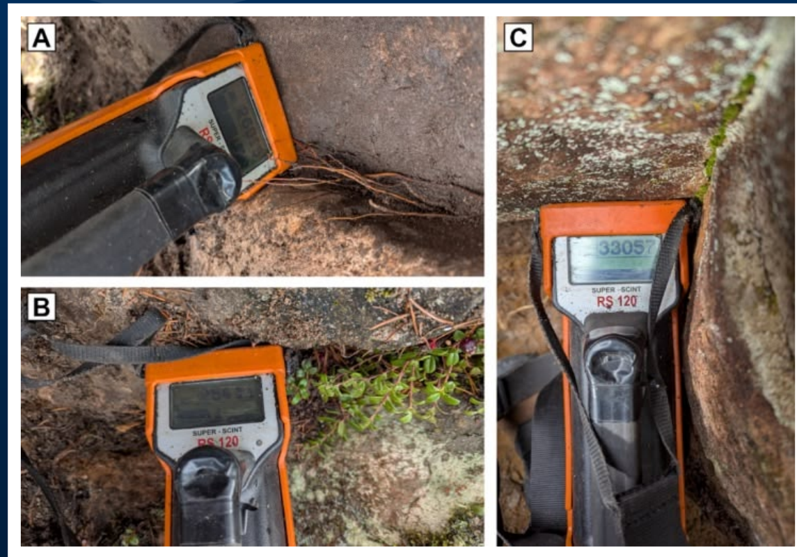
Investigation at SMDI showing 5781 (13V 416713 E, 6274629 N) returned strong radioactivity across an area of 35 m. Scintillometer readings ranging from: A) 26,900 cps, B) 25,400 cps, and C) 33,000 cps.
